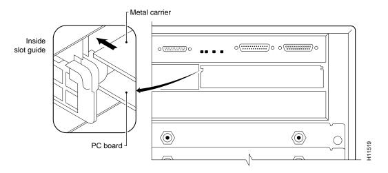
**Step 4** With the metal carrier aligned in the slot guides, gently slide the port adapter halfway into the slot.
